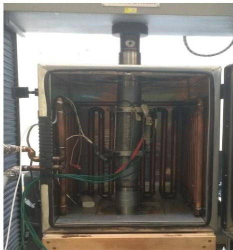
Figure 1. Test setup including cylindrical specimen made of cement paste and five Linear Variable Differential Transducers attached to the specimen using two parallel aluminum rings
